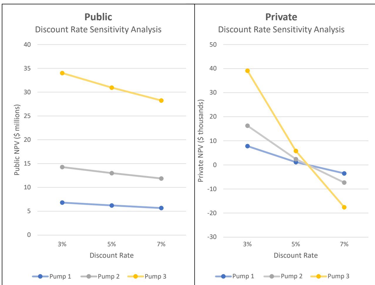
Figure 7 - Sensitivity analysis for each pump specification (1 is blue, 2 is grey, 3 is yellow) was conducted for the public (left graph) and private (right graph) NPV under varying discount rates: 3%, 5%, and 7%, ceteris paribus .
