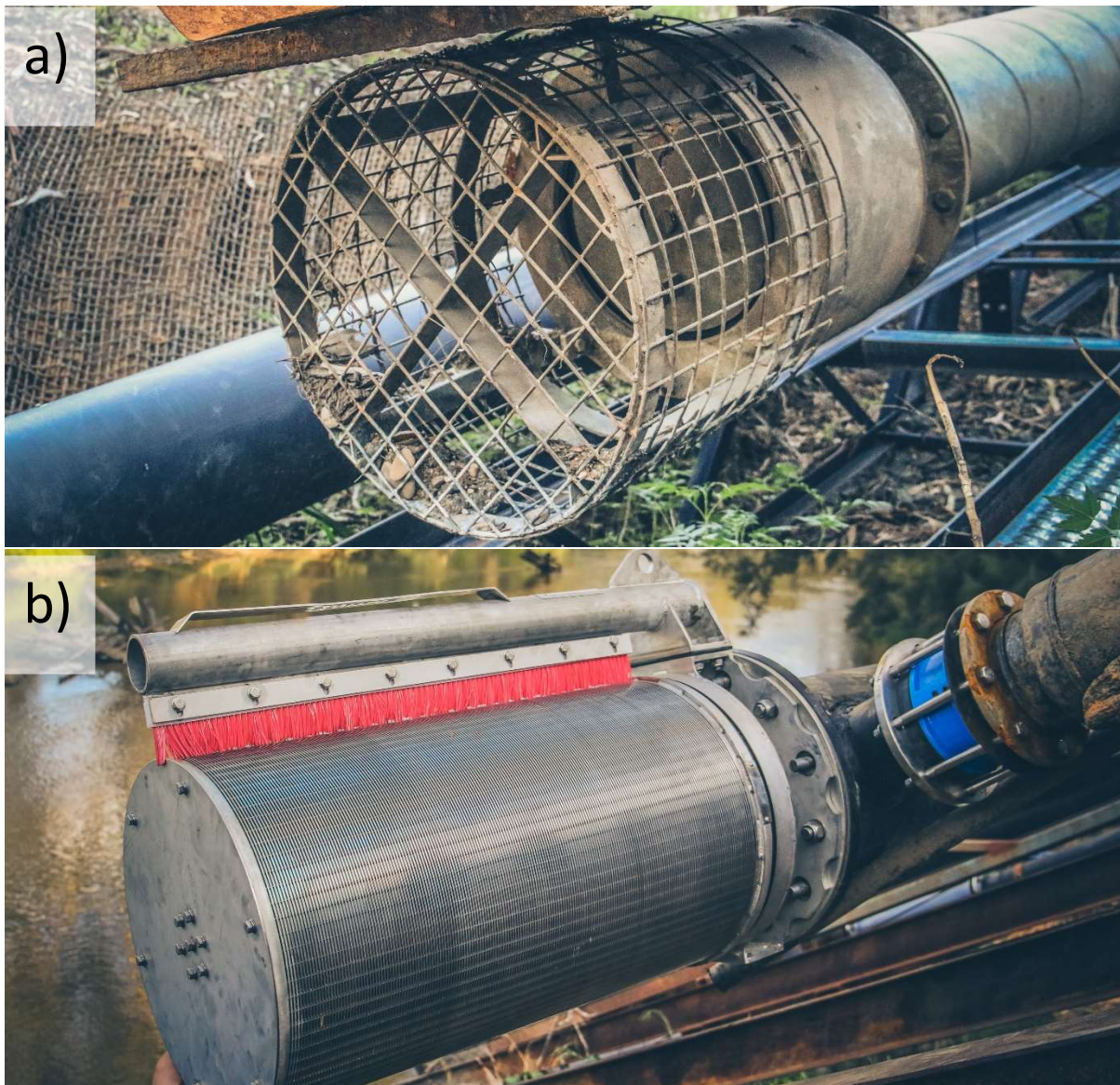
Figure 1 – Comparison of a traditional “trash rack” (a) with a modern fish-protection screen (b). Trash racks are the traditional solution to debris management in the MDB. They draw water at high velocities which can cause debris to become impinged on the rack’s surface. This can lead to fish injury or mortality and decreased pumping efficiencies for irrigators. Smaller fish, eggs, and larvae can also become entrained with diverted water through the rack’s gaps, removing them from the breeding population. Fish-protection screens draw water at lower velocities and have finer mesh, preventing fish impingement and entrainment. Some designs are even self-cleaning, further enhancing their efficiency. Images courtesy of Tom Rayner.
